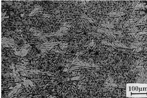
(b) \beta -quenched and aged at 773K showing hard intermetallics.
